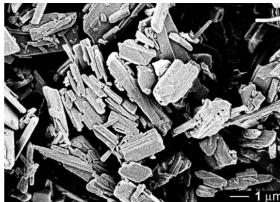
FIGURE 5. SEM image of precipitated mannitol with SDS.
